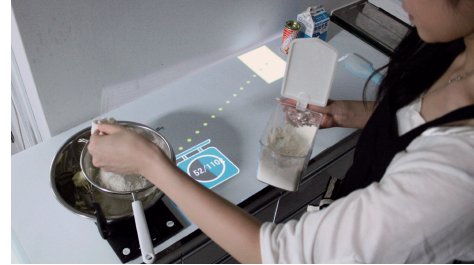
Figure 1. MimiCook system: Cooking instructions are directly projected onto the kitchen counter. Guidance information automatically changes in accordance with the user's progress.
