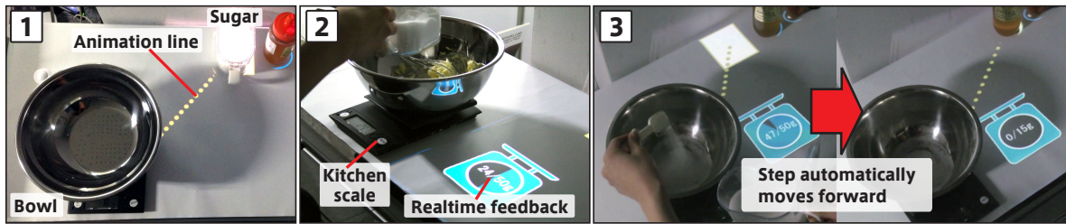
Figure 2. Main ideas. (1) Instructions are projected directly onto the kitchen counter and objects. (2) Scaling device with Bluetooth provides real-time feedback. (3) Step automatically moves forward in accordance with weights and objects' movements.
